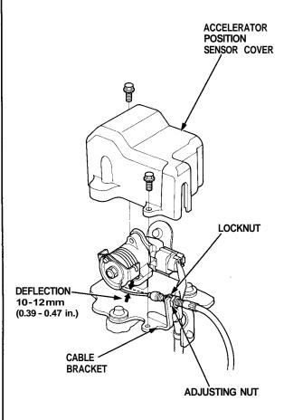
If deflection is not within specs, loosen the locknut, turn the adjusting nut until the deflection is as specified then retighten the locknut.
