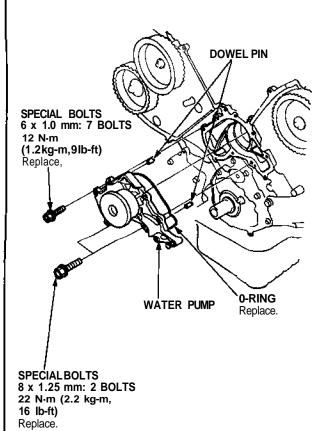
3. Install the water pump in the reverse order of removal.
