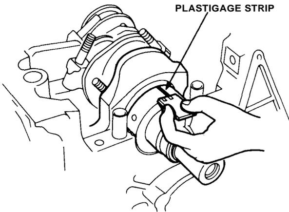
7. If the plastigage measures too wide or too narrow, (remove the engine if it's still in the car), remove the crankshaft, and remove the upper half of the bearing. Install a new, complete bearing with the same color code (select the color as shown on next page), and recheck the clearance.
