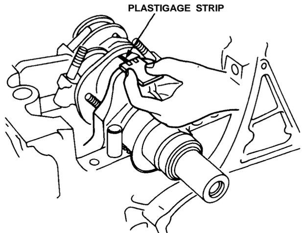
6. If the plastigage measures too wide or too narrow, remove the upper half of the bearing, install a new, complete bearing with the same color code (select color as shown on next page), and recheck the clearance.
