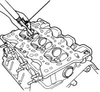
If a valve guide still won't move, drill it out with a 8 mm (5/16 inch) bit, then try again.
