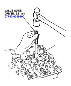
Valve Guide Installed Height: Intake: 13.75-14.25 mm (0.541-0.561 in) Exhaust: 13.75-14.25 mm (0.541-0.561 in)
