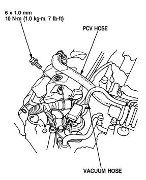
23. Remove the harness covers and ground cables from the intake manifold.
