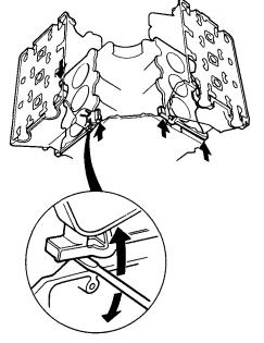
40. Remove the front and rear exhaust manifolds (see page 9-4).
