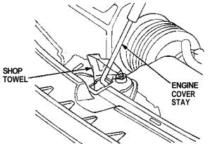
11. Relieve fuel pressure by loosening the service bolt on the fuel filter about one turn (see section 11).
