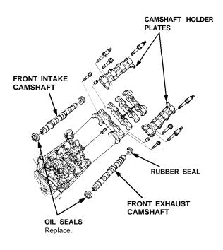
39. Remove the cylinder head bolts, then remove the cylinder head.
