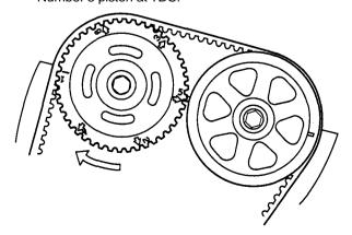
10. Rotate the crankshaft 120° clockwise (camshaft pulley turns 60°). Check that the front intake camshaft pulley is positioned as shown.
