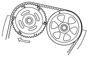
Rotate the crankshaft 120° clockwise (camshaft pulley turns 60°). Check that the front intake camshaft pulley is positioned as shown.
