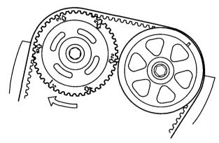
9. Rotate the crankshaft 120° clockwise (camshaft pulley turns 60°). Check that the front intake camshaft pulley is positioned as shown.
