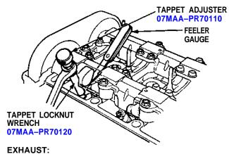
NOTE: Use a mirror to check if the special tool is positioned on the locknut correctly.
