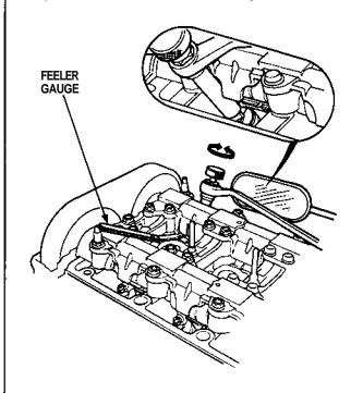
Tighten the locknut and check the clearance again. Repeat adjustment if necessary.
