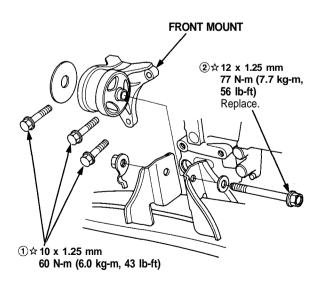
☆: CORROSION RESISTANT BOLT/NUT
