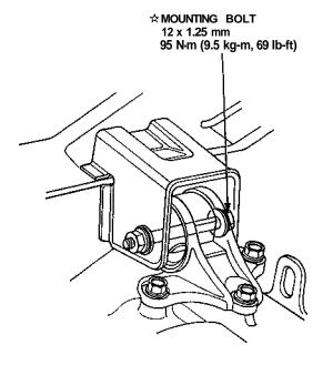
7. Tighten the rear mount mounting bolt.
