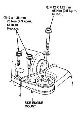
6. Tighten the transmission mount mounting bolt.
